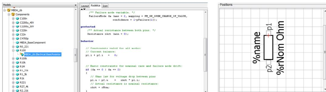
Figure 9: Physical component modeling: a) Model Library b) Code for physical model c) Graphical icon definition
