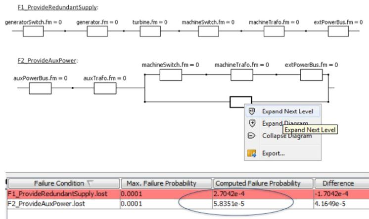
Figure 4: Results of Reliability Analysis a) Hierarchical RBD for F1 and F2 b) Comparison of failure probabilities
