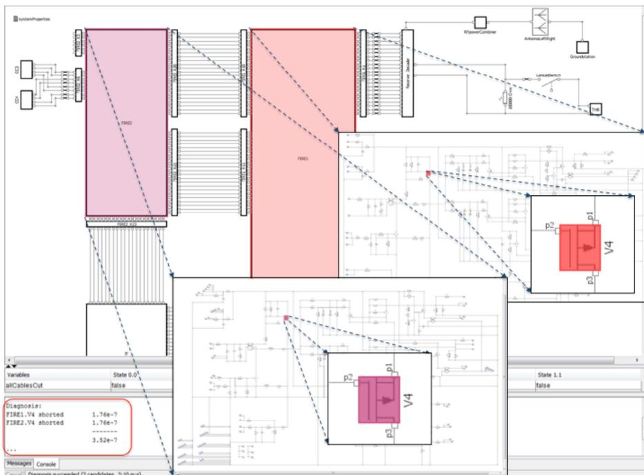
Figure 10: Hierarchical system with display of two candidates from a model-based diagnosis.
