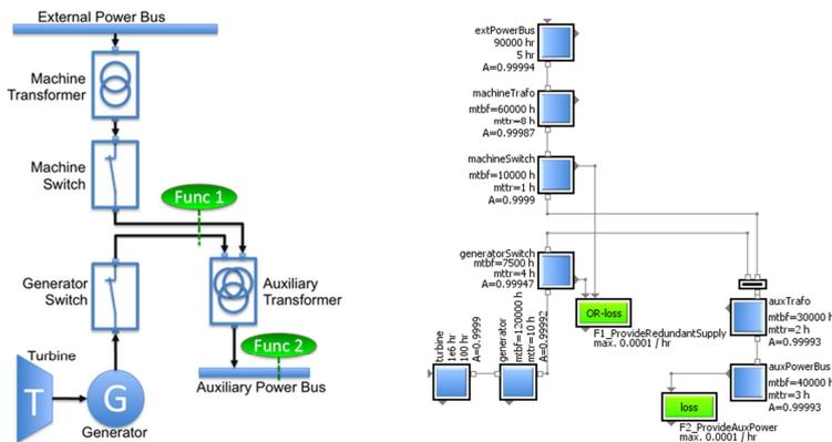
Figure 2: Auxiliary Power Supply: a) Block Diagram b) System model
