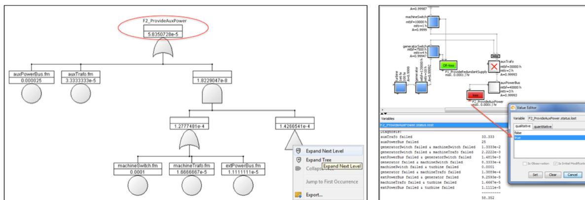
Figure 5: Safety Analyses for lost function F2 a) via Fault Tree b) via Model-based Diagnosis
